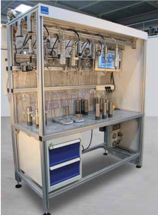
Manual measuring station for cylinder heads
