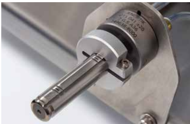
Air spindle with two elongated jets
