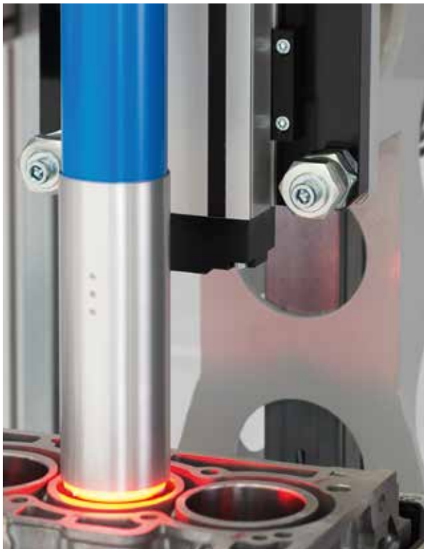
Optical surface inspection in bores
