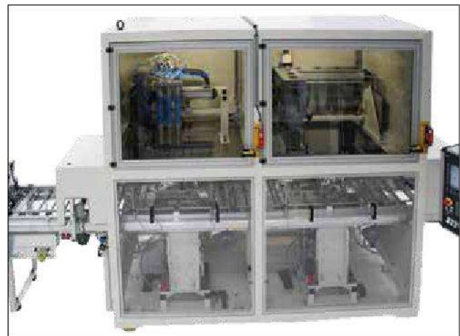
Full inspection of cylinder bore and plane surface on the engine block
